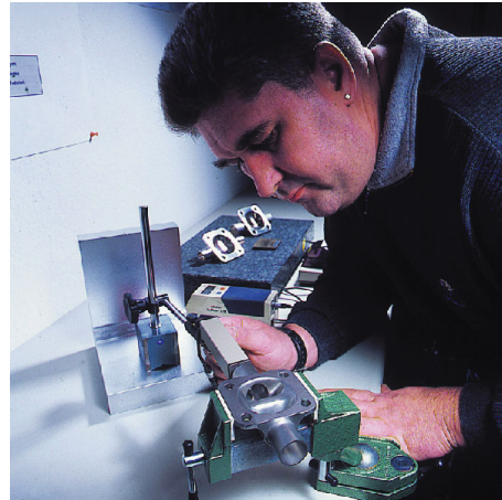
The surface finish, roughness, is measured and recorded at defined reference points according to DIN EN ISO 4287.
