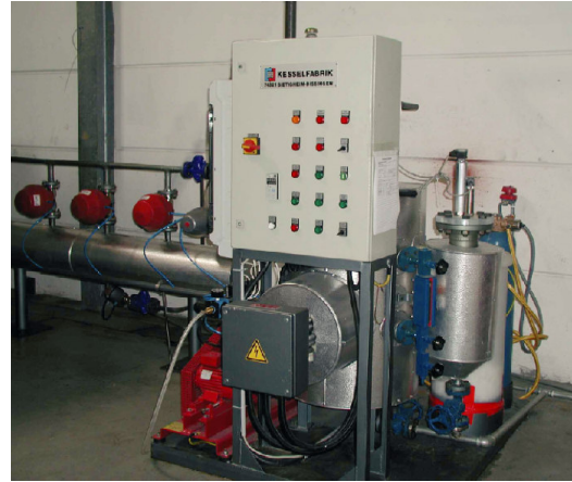
Cycle and lifetime testing of diaphragms and valves with saturated steam. Process sterilization process simulation.
