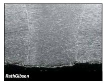
Secondary electron image of transverse section of RathGibson laser-welded 304L tubing after weld decay corrosion testing per ASTM A249-S7. Note the base-metal thinning in excess of weld thinning, as well as the lack of heat affected zone (HAZ) attack.
