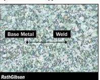
Optical image of RathGibson's 304L laser welded product with complete weld recrystallization. Note that the weld is virtually indistinguishable from the base metal.
