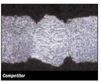
Secondary electron image of transverse section of competitor's laser-welded 304L tubing after weld decay corrosion testing per ASTM A249-S7. Photo was taken from competitor's literature. Note the unrecrystallized weld, as well as the significant attack of the fusion boundary and HAZ during ASTM A249-S7 corrosion testing.
