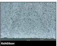
Transverse section of RathGibson laser welded 0.083" (2.11 mm) average wall tubing. The tube's ID surface is visible at the bottom. Note the weld recrystallization and the ID weld.
