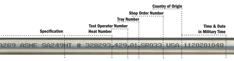
(ABOVE) Line marking is an important key to maintaining quality control and traceability. Complete product description, specifications, manufacturing and testing information are included.
